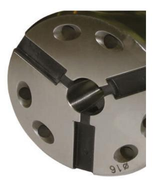
Dead Length Collets Dead length collets with single or double cone
